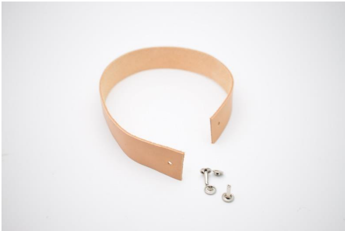
15. Cut your leather strap to size and make holes in the ends for the rivets.
