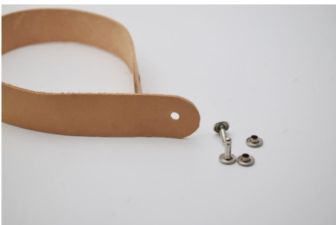
Cut the leather strap so you have a piece that is approx. 14 ½", rounding the corners slightly. Using the leather punch, make a hole on either end.
